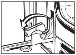
■ Flip down the locking clamps on each door hinge.
